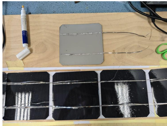
Figure 10 – Series connection through tabbing soldering
