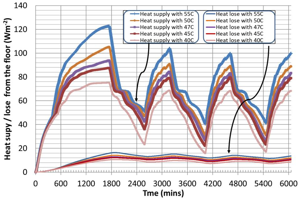
Figure 7 Heat supply from the floor surface to the room and lose from the bottom of the floor under different water inlet temperatures
