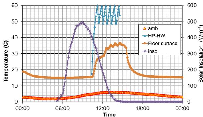
Figure 3. Predicted floor surface temperature using the realistic hot water supply from heat pump running under the local ambient conditions in 24hrs
