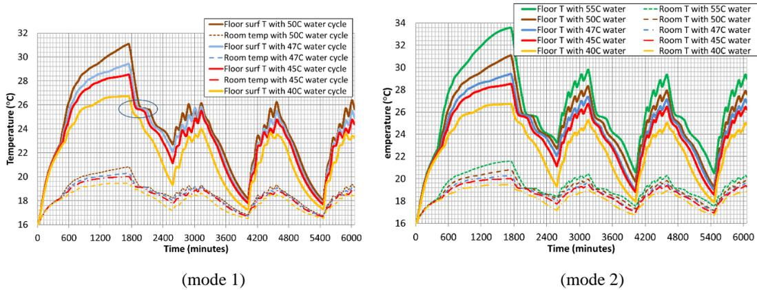
Figure 4 Floor surface temperature and indoor room temperature variation with different water inlet temperatures under mode 1 and 2 operations
