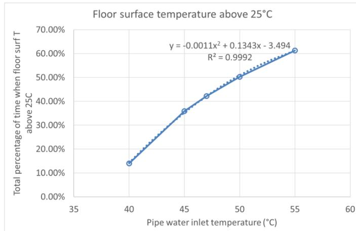
Figure 9 The total percentage of the time when the floor surface temperature is above 25°C in each day with five difference hot water inlet temperatures of 40, 45, 47, 50 and 55°C
