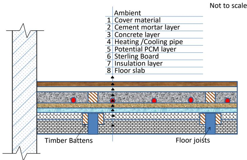
Figure 2. A schematic diagram of underfloor heating system structure with potential layers and joists (Huang et al., 2015)
