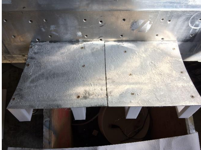
Figure 5. 10 Gluing process for small CPC systems
