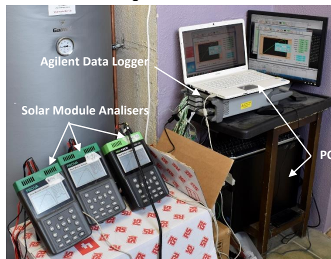
Figure 7. 18 Systems installed at Brackloon Drummin Community Centre façade in Mayo. The front wall has a deviation of 46^\circ with the south. The outdoor experimental performance of the systems was monitored using three independent solar module analyzer, Agilent data logger, Kipp and Zonen Sp Lite 2. The details of these devices were described in section 3.5. All the data were recorded every 2 minutes. The solar module analyzers and Agilent data logger were linked to a PC as shown in figure 7.19.
