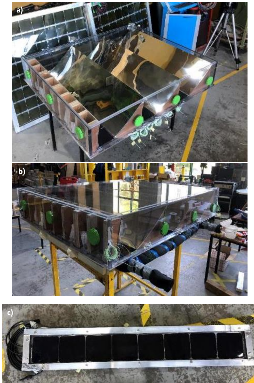
Figure 6. 31 Mayo Final system assembly (a) CPC system (b) CPC/PCM system (c) Reference system
