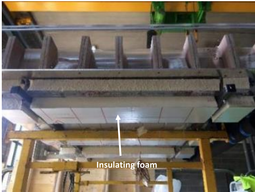
Figure 6. 21 Insulation installed in the PCM containers
