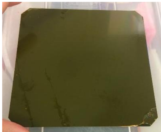
Figure 3. 5 One Luminescent down shifting layer (LDS)
