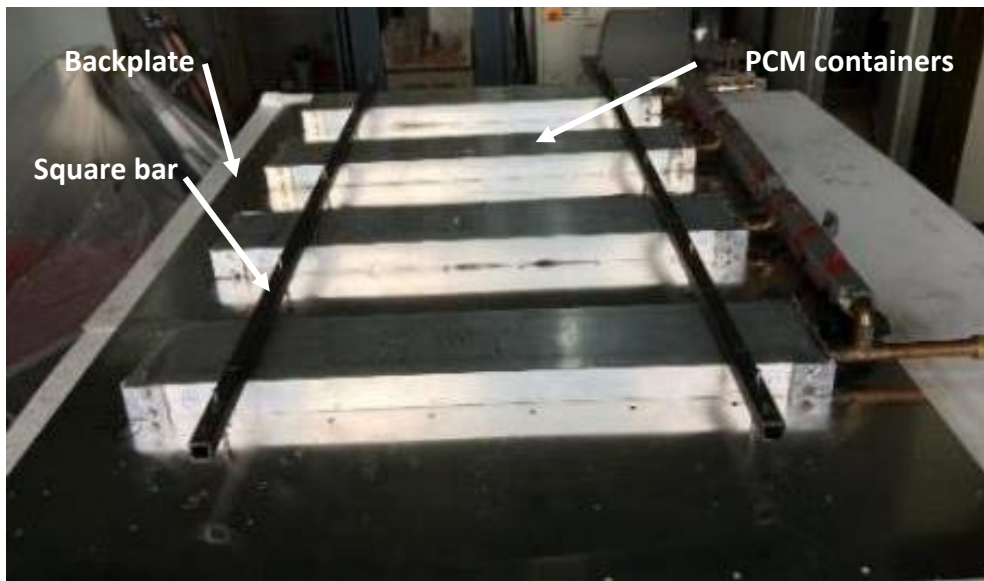
Figure 6. 19 PCM containers installed in the backplate
