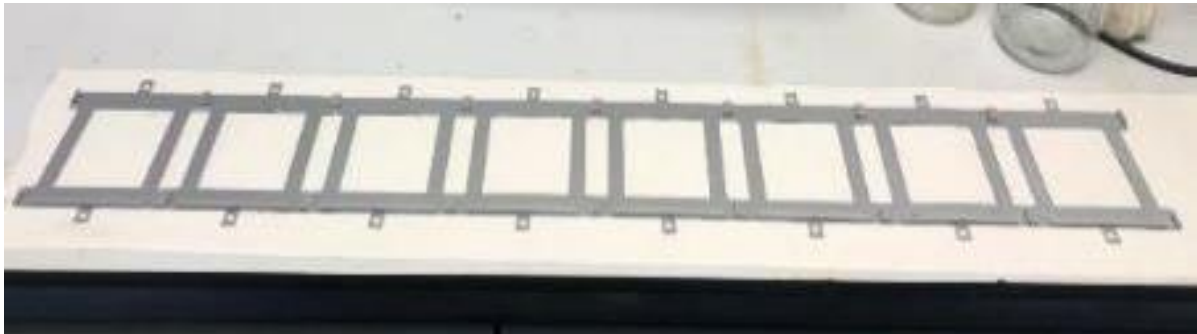
Figure 6. 6 Full string of eight solar cells holders
