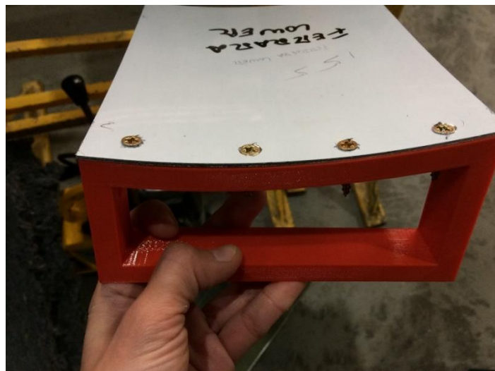
Figure 5. 9 Auxiliary plates installed on the reflector support
