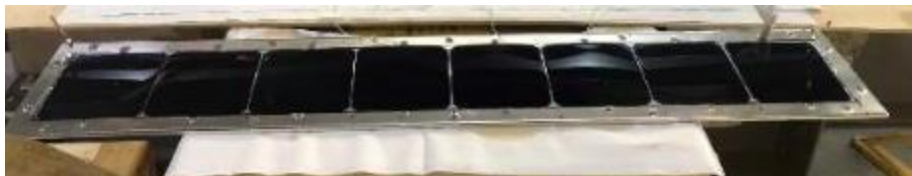
Figure 6. 29 Reference system with solar cells encapsulated
