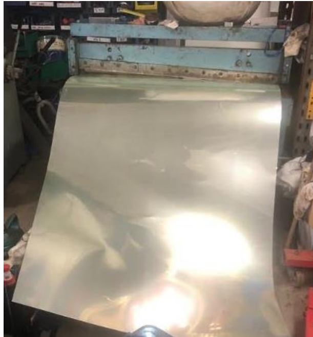
Figure 6. 9 Guillotine used for cutting Alanod reflectors
