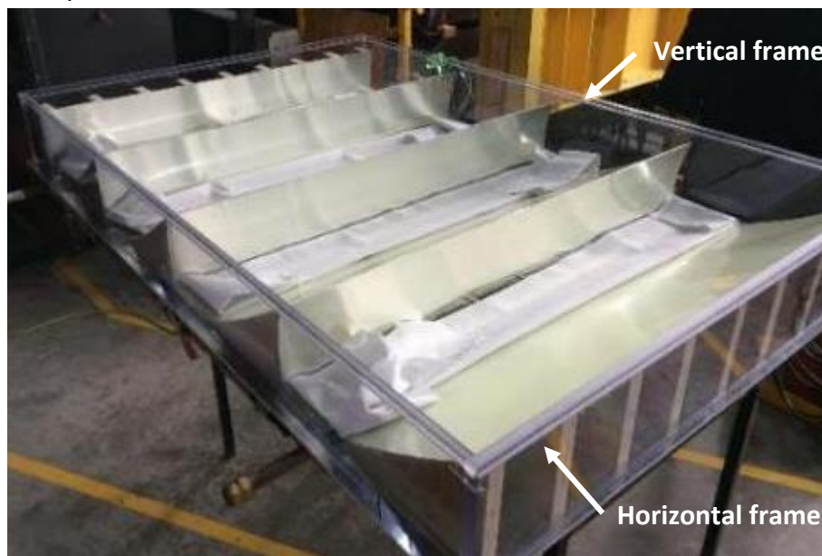
Figure 6. 17 Frame installed in the CPC System
